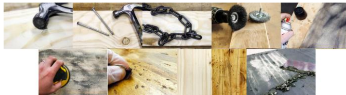
Figure 7. Distressing & Wire-brushing process Source: Mikesaurus, 2019
