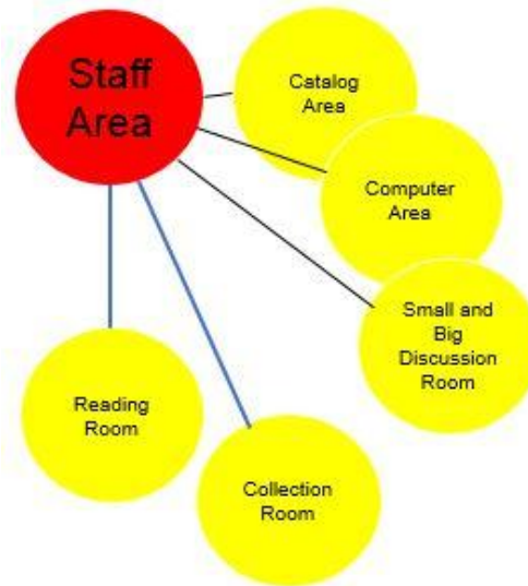
Diagram 1 Relationship Between Nearby Zones (black line: close; blue line: moderate to far)
