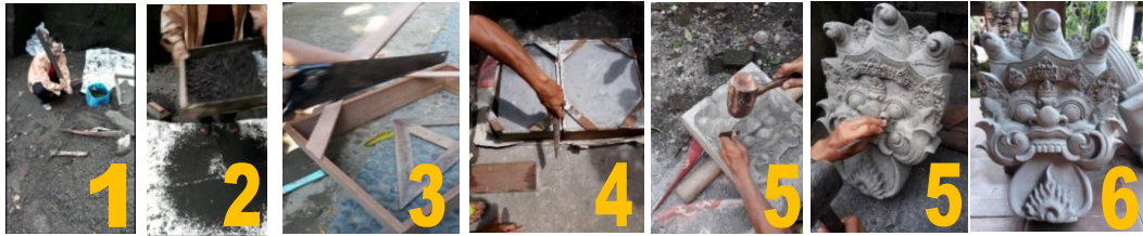
Figure 2. (1) taking crumbs of used solid stone; (2) sifting; (3) making molds; (4) fabrication; (5) carving; (6) final result Source: Pranajaya (2020)
