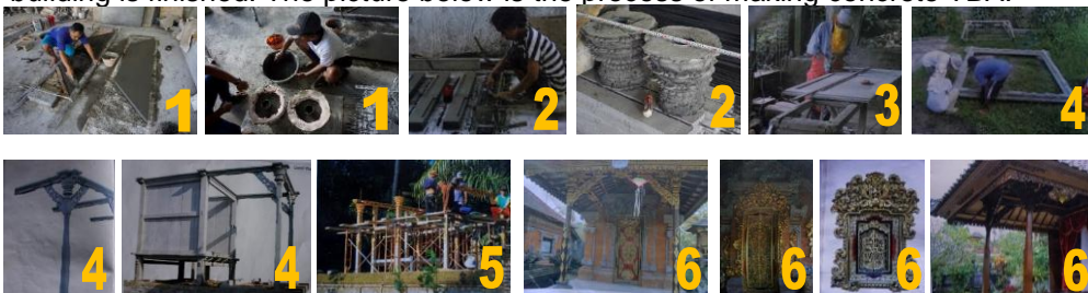
Figure 4. (1) Pouring dough to the mold; (2) open the mold; (3) smoothing; (4) assemble; (5) install roof trust; (6) applied result Source: Pranajaya (2020)
